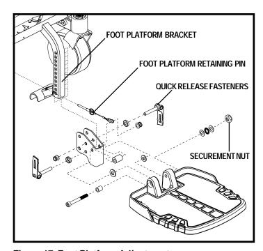
Figure 17. Foot Platform Adjustment
